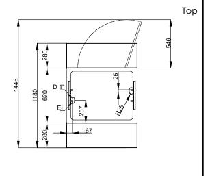
Electric Supply voltage: 220-240 V/1N ph/50/60 Hz Electrical power, max: 2.32 kW Water: Drain line size: 3/4" **Key Information:** N° of doors: External dimensions, Width: 800 mm 1180 mm External dimensions, Depth: External dimensions, Height: 1304 mm Net weight: 97.5 kg Shipping height: 1334 mm Shipping width: 840 mm Shipping depth: 899 mm Shipping volume: 1.01 m<sup>3</sup> +85 / +9<u>5</u> °C Set temperature:
